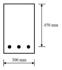
As per Limit State Design of IS 456:2000, the design moment capacity (in kN.m, round off to two decimal places) of the beam section, is \_\_\_\_\_\_.
