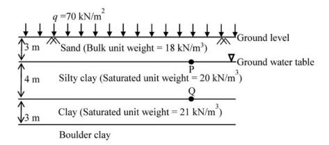
Immediately after preloading, the effective stresses (in kPa) at points P and Q, respectively, are
